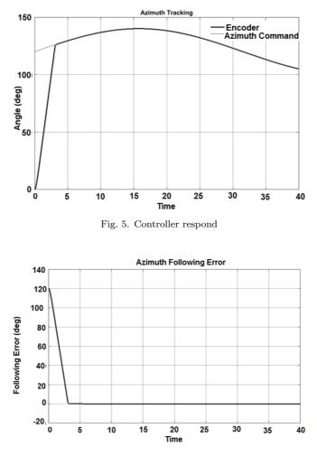
Fig. 6. Controller tracking error
